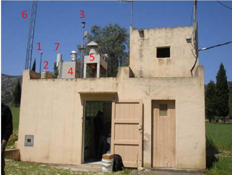
Figure 1.10. 1) Inlet for gaseous sampling ( \text{SO}_2 , \text{NO} , \text{NO}_2 , \text{O}_3 ) with conventional instrumentation; 2) Grimm optical particle counter ( \text{PM}_{10} , \text{PM}_{2.5} , \text{PM}_1 ); 3) Inlet for the beta absorption monitor; 4) Sequential high-volume \text{PM}_{10} sampler; 5) Automatic collector of dry and wet deposition; 6) meteorological tower (temperature, relative humidity, pressure, wind direction and velocity); 7) rainfall collector.
