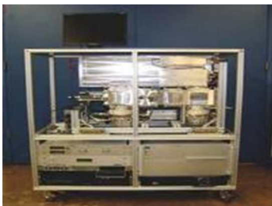
Figure 5.3. On-line aerosol analysis methodology: Highly time-resolved on-line measurements of particle composition were performed using an Aerosol Mass Spectrometer (HR-ToF-AMS).
