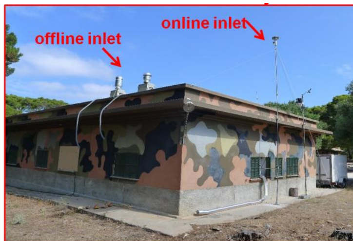
Figure 1.13. Es Pinar Cape off line inlets indicated on the left site and on line measurements inlet on the right side.
